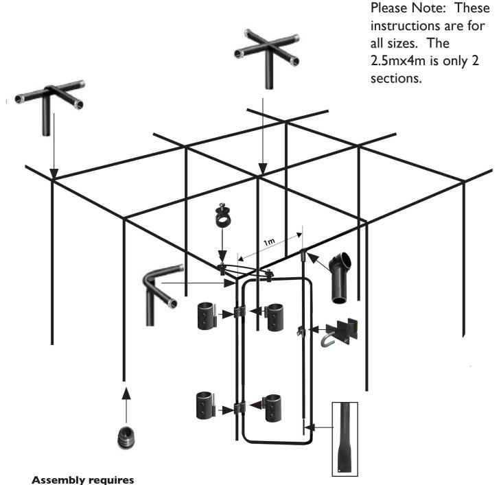
Rubber Mallet, an Allen Key (Provided) a Philips head Screwdriver, Spirit Level, Scissors and Tape Measure.
