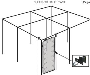
8. Drop the completed door onto the hinged on the door upright. Adjust hinges on the upright as required.
