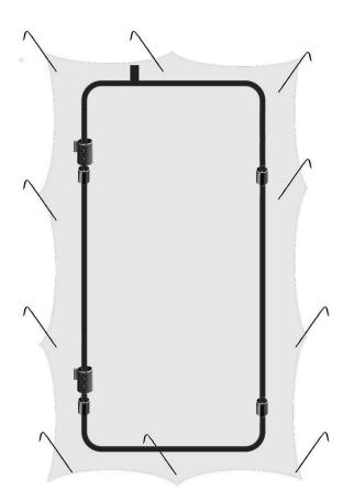
**2.** Cut out a section of the side net just larger than the door and stretch out with ground pegs.
