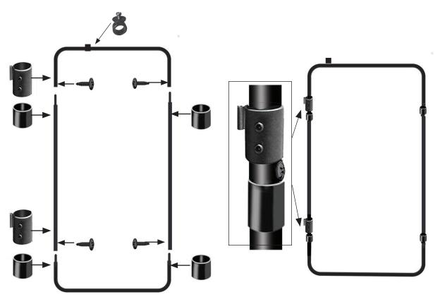
**1.** Lay the door frame parts out. Thread 2 moisture seals below the joins on either side of the door. Thread door hinges above the joins on one side.
