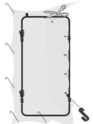
**4.** As you remove the ground pegs trim the net leaving just enough to fold the excess net over the frame. Attach with S Hooks. Complete the process a.nd then put the door to one side.
