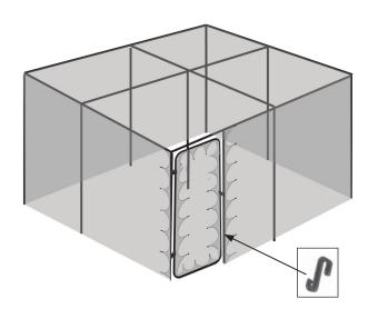
**9.** Attach the side net to the perimeter cross bars with cable ties and to the door uprights with 'S' Hooks.
