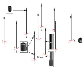
6. Drive a hole to the depth marked on the hole-maker which is approx. 38cm – the easiest way to do this is by placing a small plank of wood over the top of the hole-maker and using a rubber mallet to hit into the ground. Insert an end plug into the base of each upright and a moisture seal at the top. Push the uprights into the ground. Make sure the pre-drill hole, on the door catch upright, is at right angles to the frame.
