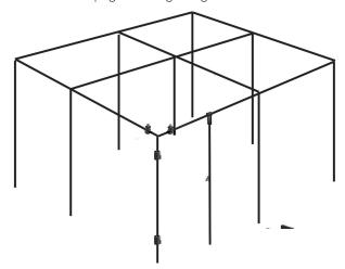
7. Place the roof on top of the uprights. Push all the moisture seals over the joints
