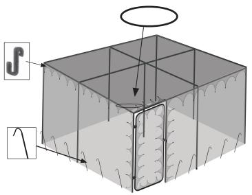
10. Attach roof net over the roof using S Hooks. Secure the side net to the ground with ground hooks. place the band on the band collars.
