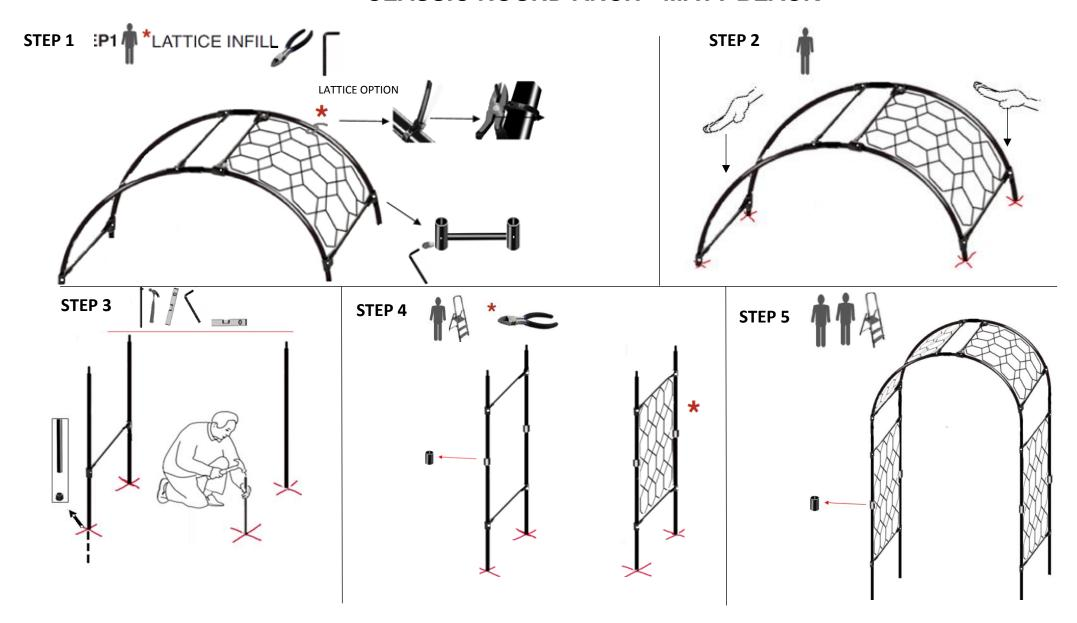
ONLY FOR ORDERS WITH LATTICE PANELS. PANELS CAN BE ORDERED FROM www.agriframes.co.uk
